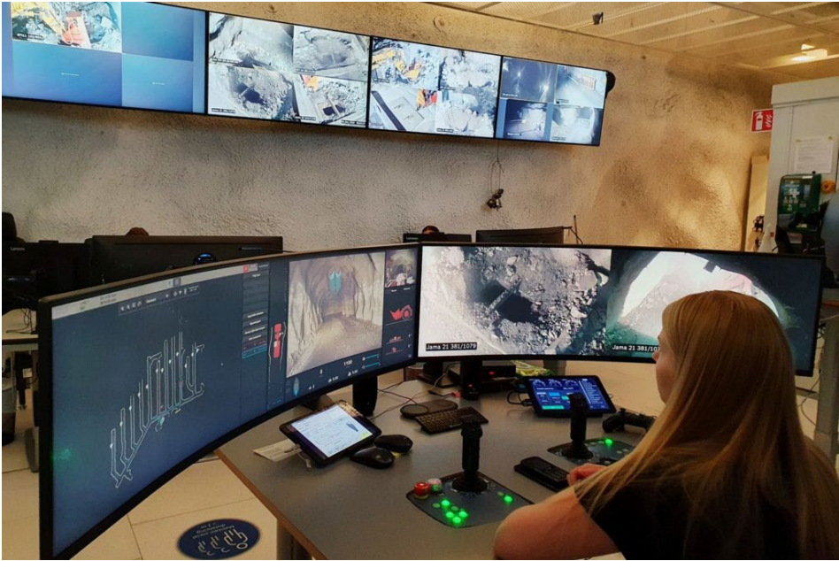
Figure 10: Underground control station of semi-autonomous LHDs at Kiruna mine [143]
