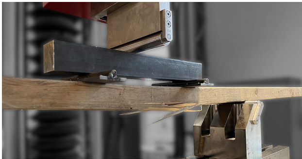
Fig. 8 Failure initiation in the proximity of a knot at the bottom surface during flat-wise bending
